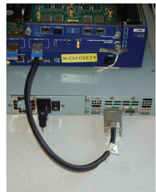
Figure 5: Appropriate Test Setup: 1) Signals are sent over a single cable, 2) the cable is a minimum length (short), and 3) the cable is properly shielded and rated for 6 Gb/s use.
